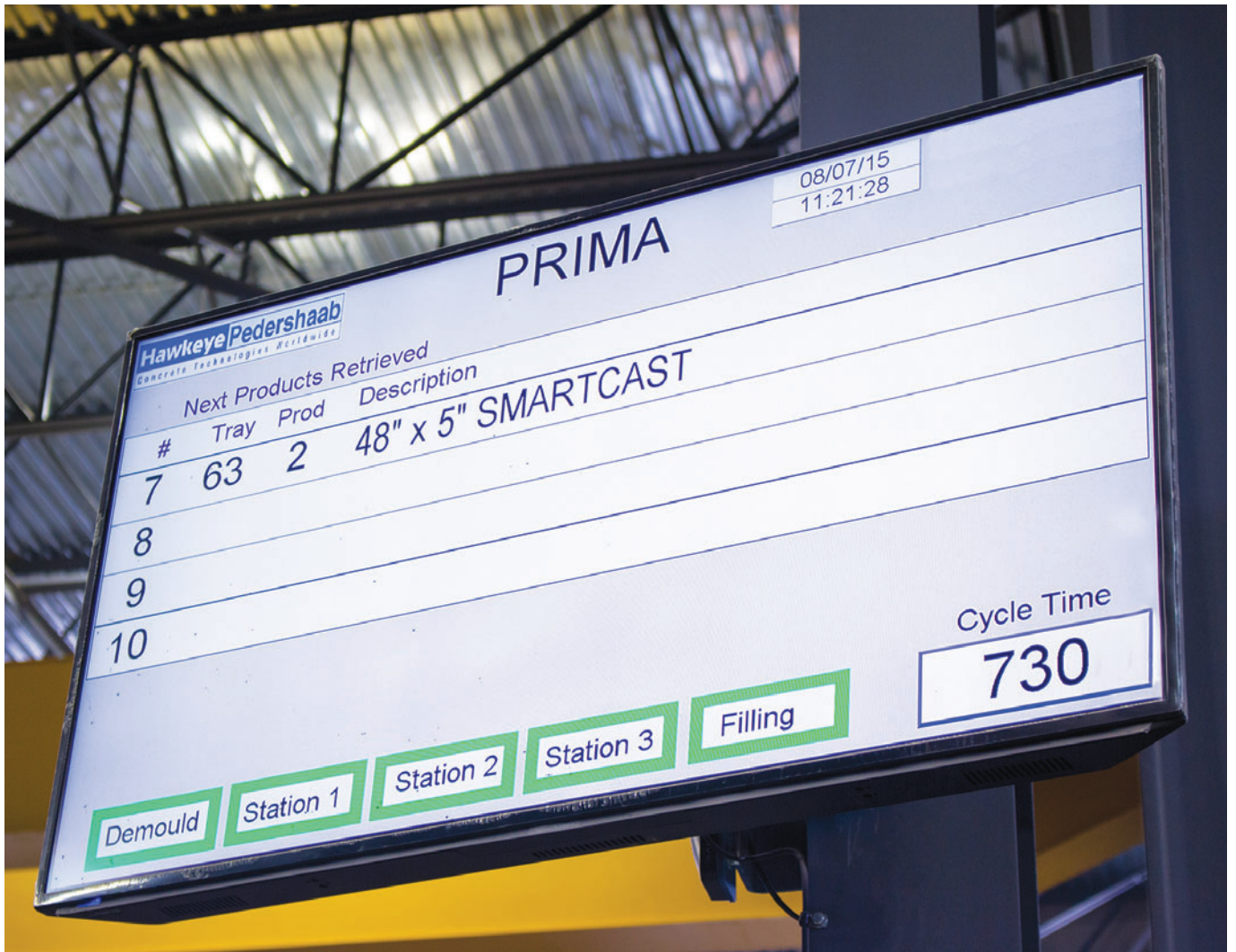
One of the advantages of Prima is its ability to build a “smart” production queue utilizing data inherent to each form.
