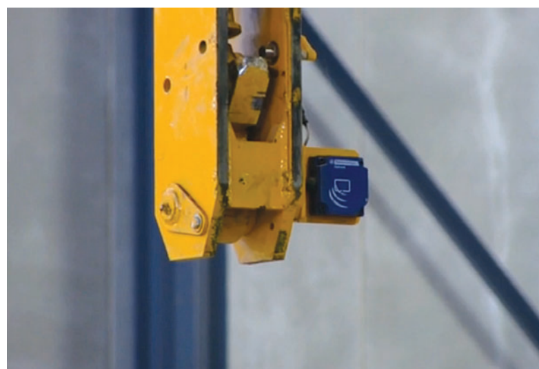
RFID reader system for form identification.
