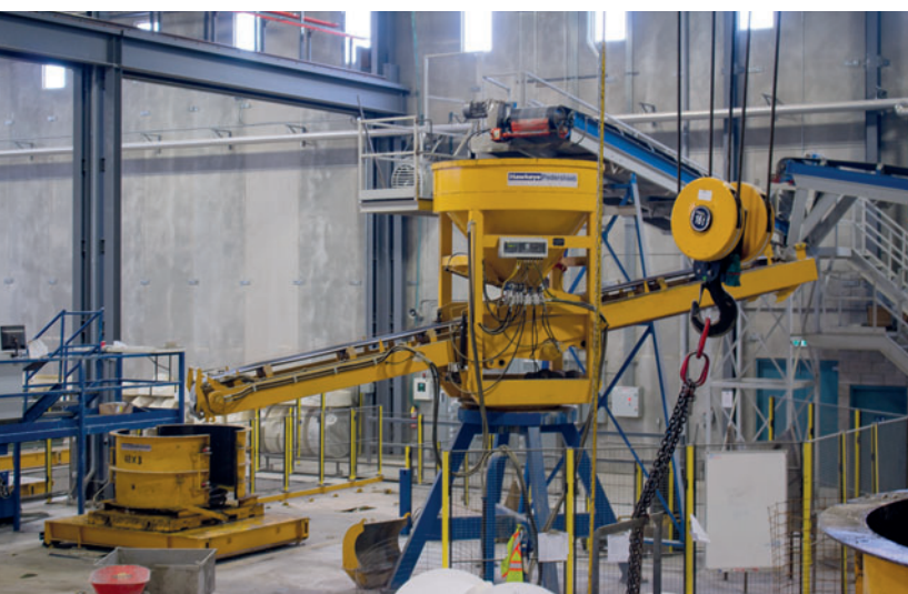
The form filling station can be configured in numerous ways, including with concrete conveyor belt, with concrete pump or with concrete bucket.
