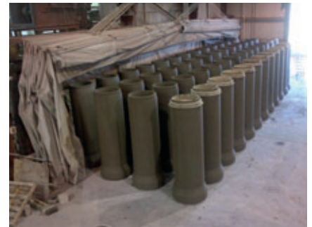
Figure 3: Here, 30-inch "green" pipe is placed in the curing area. A fabric curing tent will be deployed to control the curing process.
