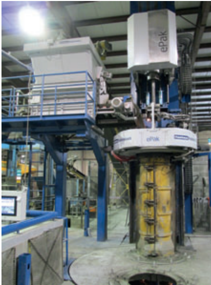
Figure 6: The new HawkeyePedershaab ePak packerhead pipe production system at Coastal Pipeline Products in Calverton, N.Y., is used to produce from 12 to 36 inch inside diameter dry cast pipe. The ePak system features a uniframe structure that eliminates the multiple support legs found on conventional systems, direct drive permanent magnetic motors provide gearless operation for greater torque and accuracy, and closed-loop PC-based controls.
