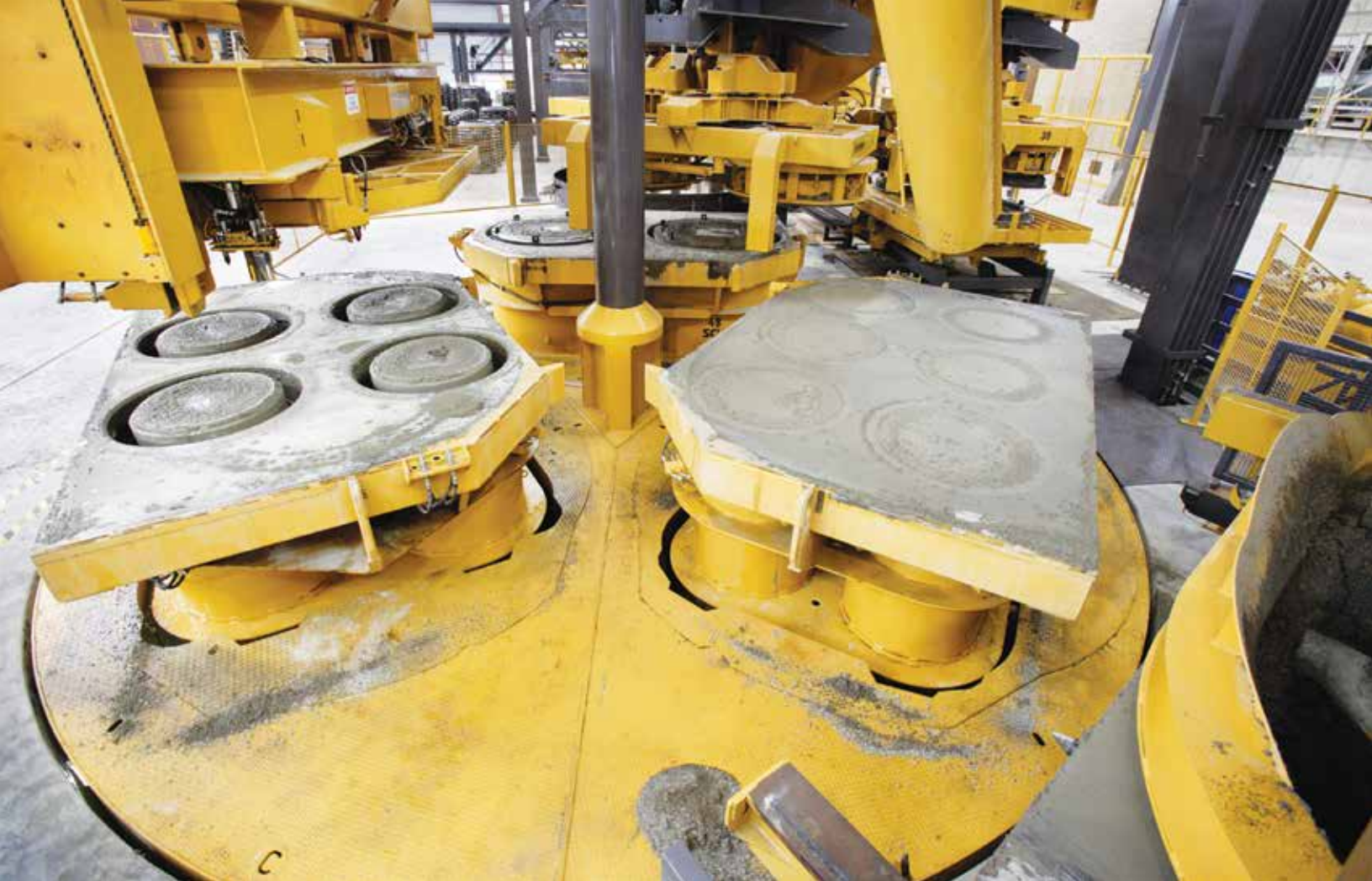
Automatic Crane Demolding
