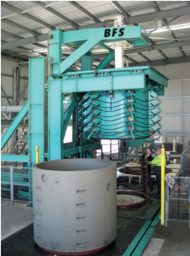
With the soakwells, the recess blockouts are withdrawn hydraulically before the demoulding process.
