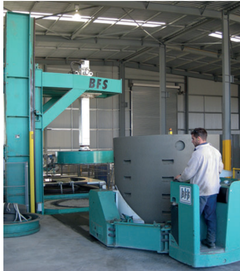
After ejection of the concrete product from the machine, employees drive it to the drying area on an electric extraction cart.
