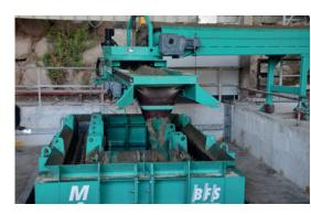
Mammut production with rotating discharge belt and CNC path control.
