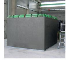
Box culverts after demoulding, with the Finitec spigot-end mould still in place.
