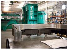
Finitec spigot-end mould for precise, clean joints
