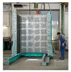
Assembly of precisely shaped modular mould parts.
