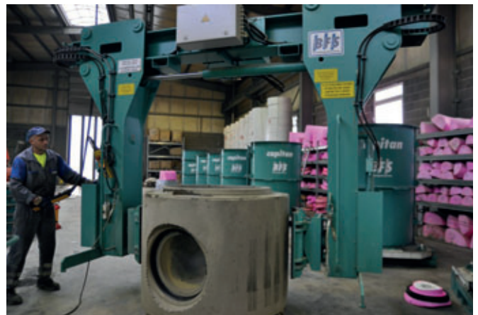
The manhole bases are safely demoulded and rotated into the installation position using the hydraulic turnover spreader beam.
