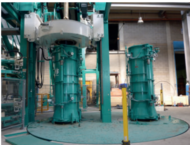
The Souveraen S 1230 has a fully revolving spigot end shaper and a weight-dependent compaction controller.
