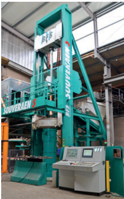
The BFS Souveraen S 1230 high-performance pipe-making machine was optimised for Chaux de Contern in order to achieve an even higher production output.
