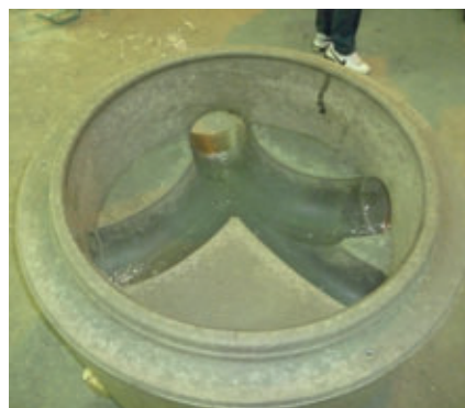
Finished Capitan manhole bottom
