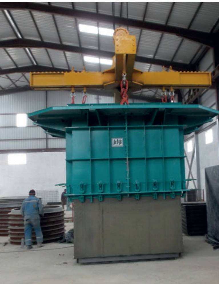
Demoulding even in confined spaces
