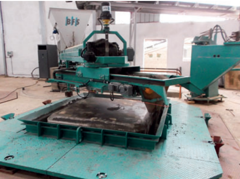
With the Jumbo 3625, pipes of different diameters or pipes and rectangular pipes can be produced in one shift.
