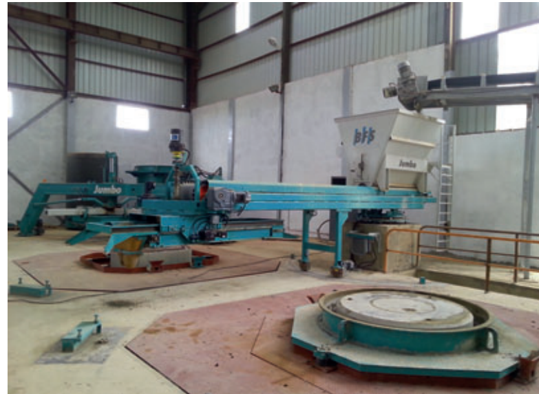
The Jumbo 3625 Duo works almost simultaneously in both working stations.
