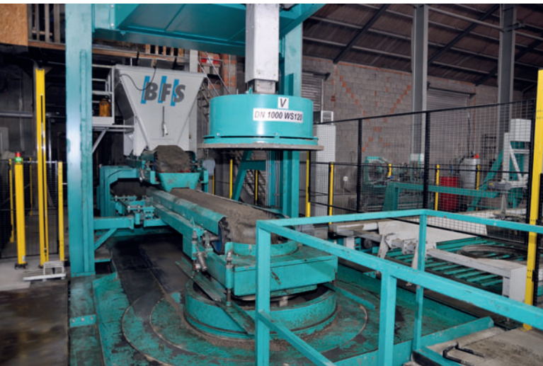
Stationary concrete silo with additional conveyor belt
