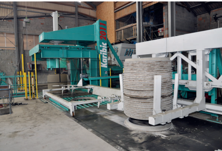
The Karibic 2011 system has been equipped with a pallet magazine with a fully automated pallet placement fixture.
