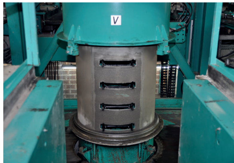
Mould core with hydraulic plate for the production of manhole rings with manhole steps
