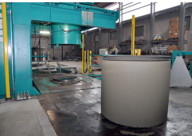
The finished products are pushed out of the machine automatically.
