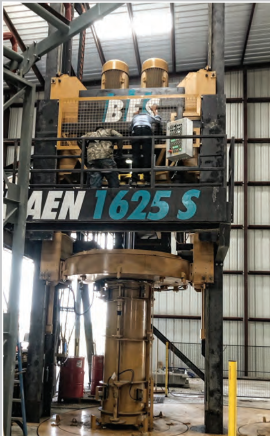
The BFS Souveraen three-piece "Power Jacket" form is an automated feature that increases efficiency and safety.
