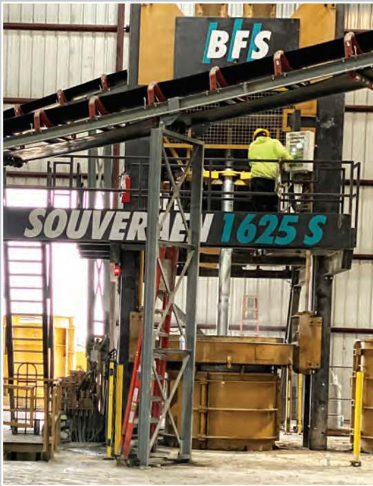
The BFS Souveraen is a fully automated concrete pipe machine for high-output production.
