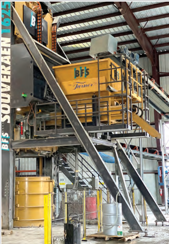
The Souveraen's counter-rotating, roller-head, compaction tools compact the concrete and are controlled by an advanced, high-tech control system.
