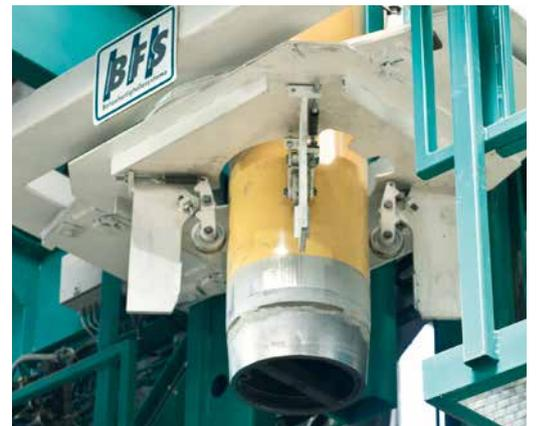
ECORESIST By the combined control of the pipe machine and liner installation the stepping order of the system is perfectly interlocked. As soon as the mould with the green pipe rotates to the insertion station, the polymer pipe is pressed in from the top.
