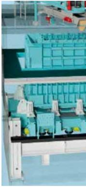
With stable hydraulic clamping jaws, the jacket (including base pallet) is braced to the vibrating table...
