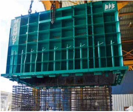
The prepared reinforcement cages on the base pallets are collected via crane by the mould jacket and placed into the system over the core.
