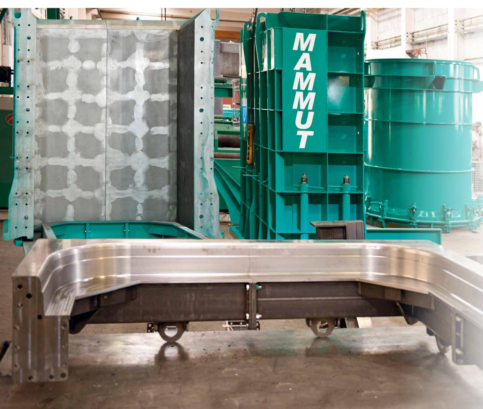
Mould cores, jackets, base pallets, spigot end shapers – all these elements belonging to the modular system reduce investment costs and increase production flexibility. MAMMUT moulds can be equipped with:
