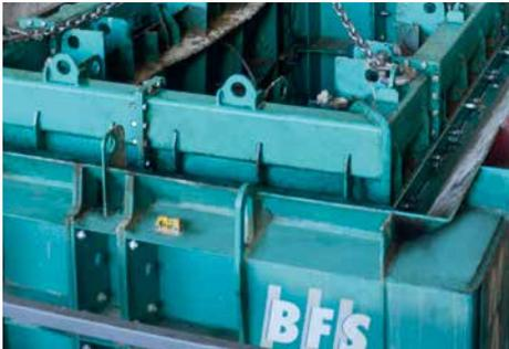
Customised designs are available for the spigot end. The spigot end is shaped under vibration, by eight hydraulic clamping cylinders integrated in the core. This production step is also completely automated. All parameters can be selected via the integrated touch screen.
