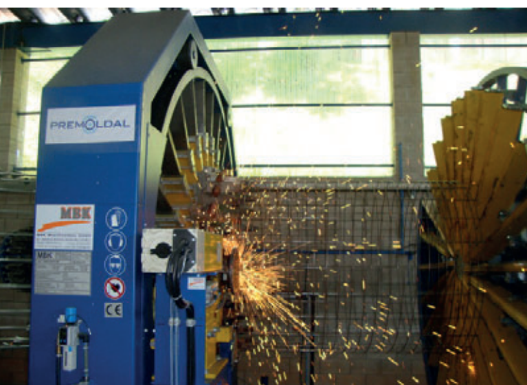
The BSM-250-R welds a wire cage
