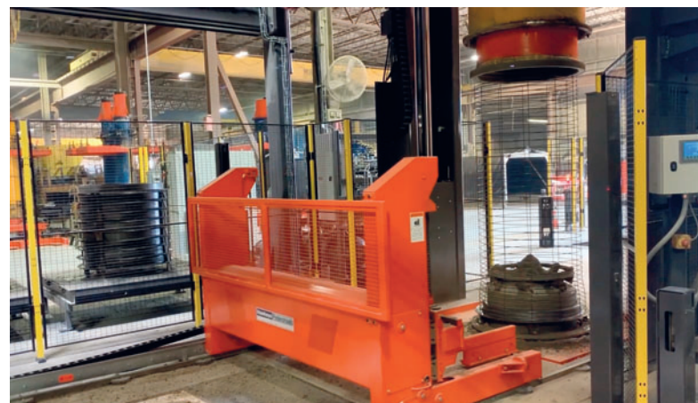
Pallet cart delivering the pallet and cage to the Mastermatic machine.
