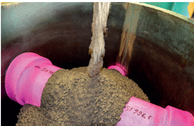
The moulds are filled by a dosing system that is operated via the bridge crane
