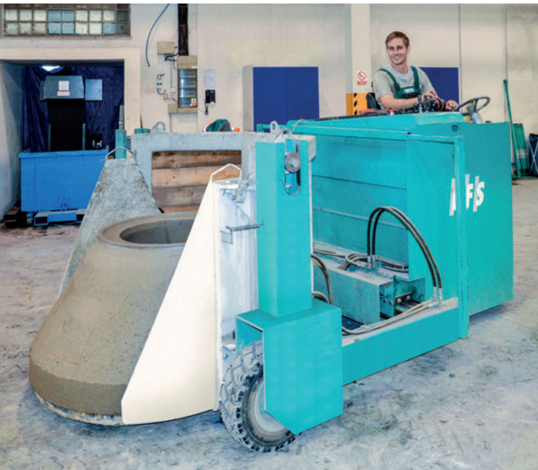
The electronic run-off truck from BFS for the removal of the products
