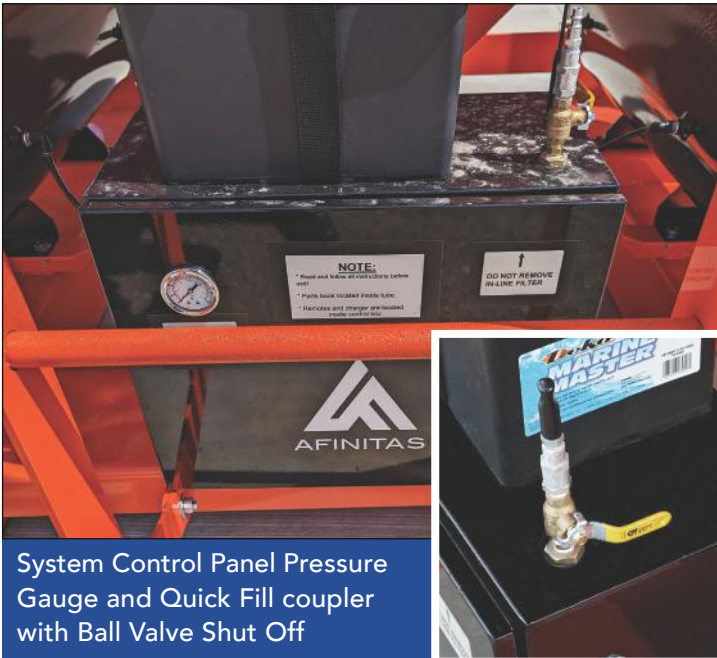
On-Board Manual Operation Valves (this is a redundant feature if electrical failure of any type should occur)
