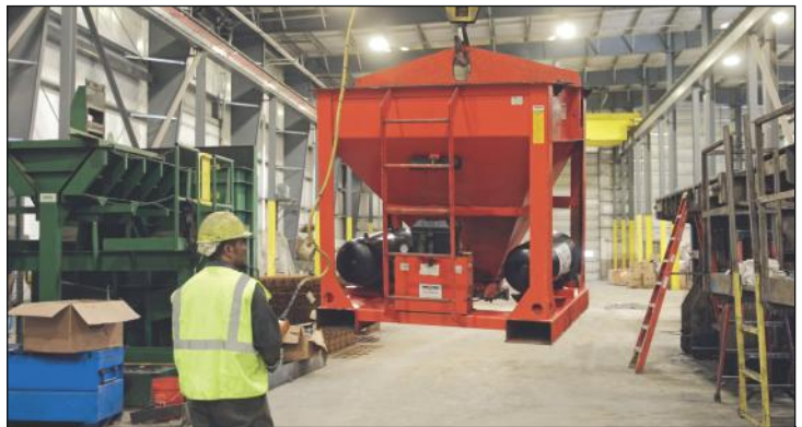
Above- Crane operator moving the Crete Hawg into position to pour forming. Below, bucket transport
