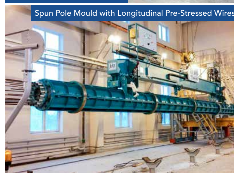
Spun Pole Demoulding Process
