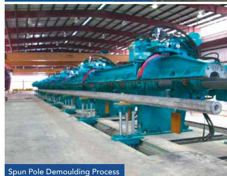
Spun Pole Mould with Longitudinal Pre-Stressed Wires
