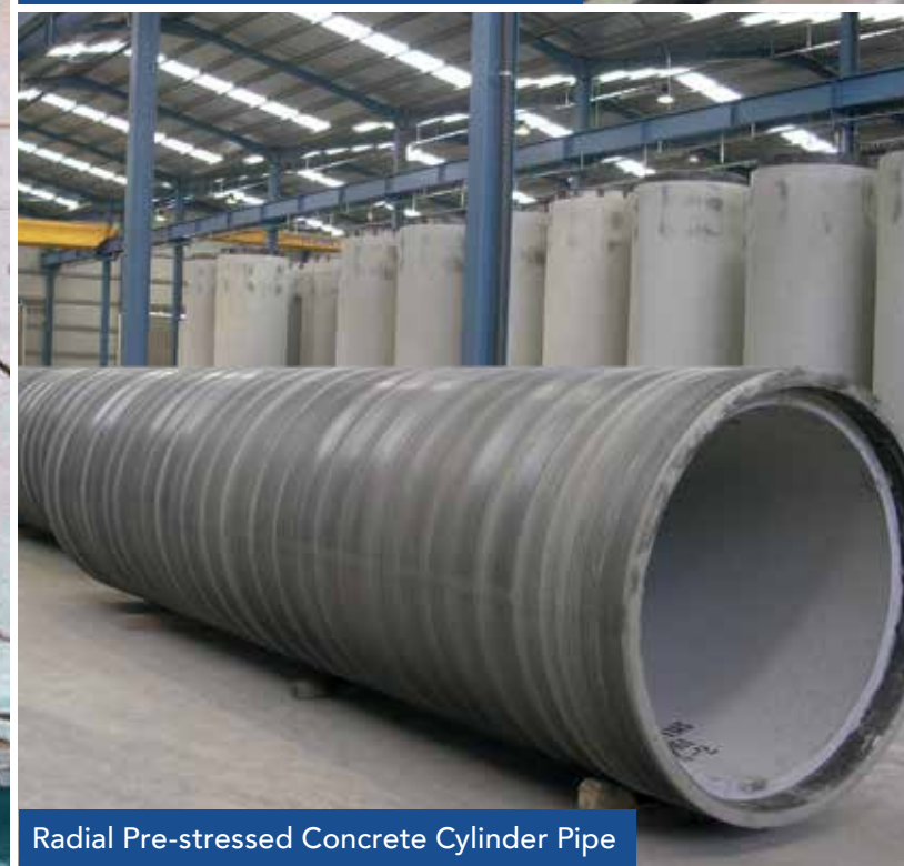
Core pipe circumferential prestressing
