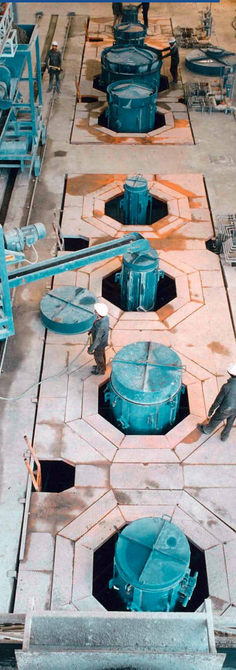
Systems for pre-stressed Steel Cylinder Pipes (PCCP) – mould filling process
