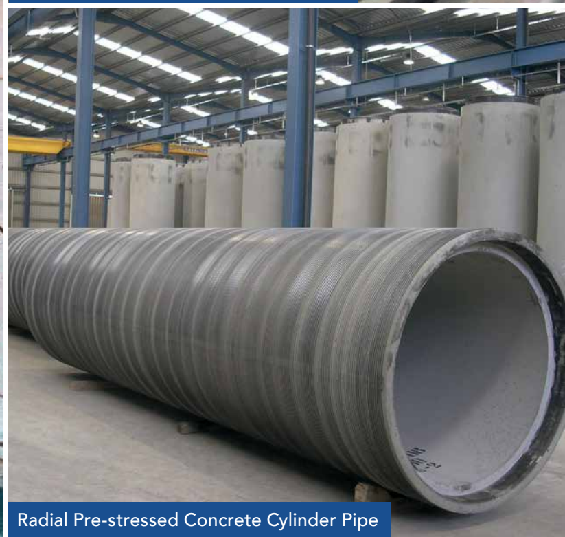
Core pipe circumferential prestressing
