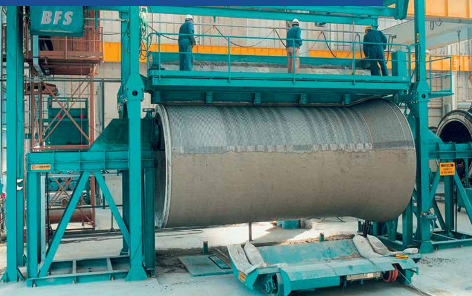
Systems for pre-stressed Steel Cylinder Pipes (PCCP) – Mortar Coating Machine; in order to protect the steel wires against corrosion
