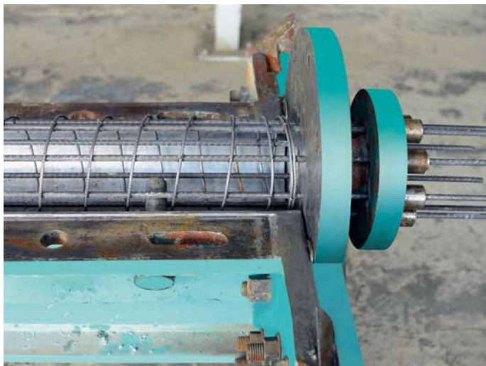
Spun Pole Mould with longitudinal pre-stressed wires
