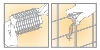
For fast installation, E-Z Klip spacers are prealigned and packaged on convenient handling strips. The E-Z Klip snaps on by hand. No tools, cutting, or welding is required.
