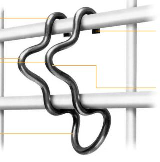
Extra long hooked ends with a generous radius to fully wrap and securely fit heavy gauge wires. Guards against spacer popping or twisting off when struck or slid over packerhead jacket splices. Note: Also available with hooked ends that fit larger diameter wire or layered cage assemblies.
