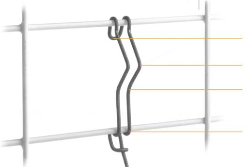
Long hooked ends securely wrap around circumferential wires. Resists pop-off or dislodgement of spacer if twisted.
