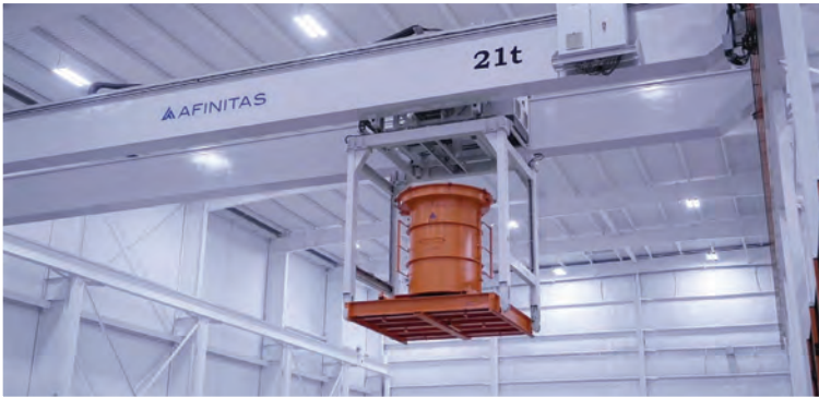
Prima's automatic overhead manipulator.
