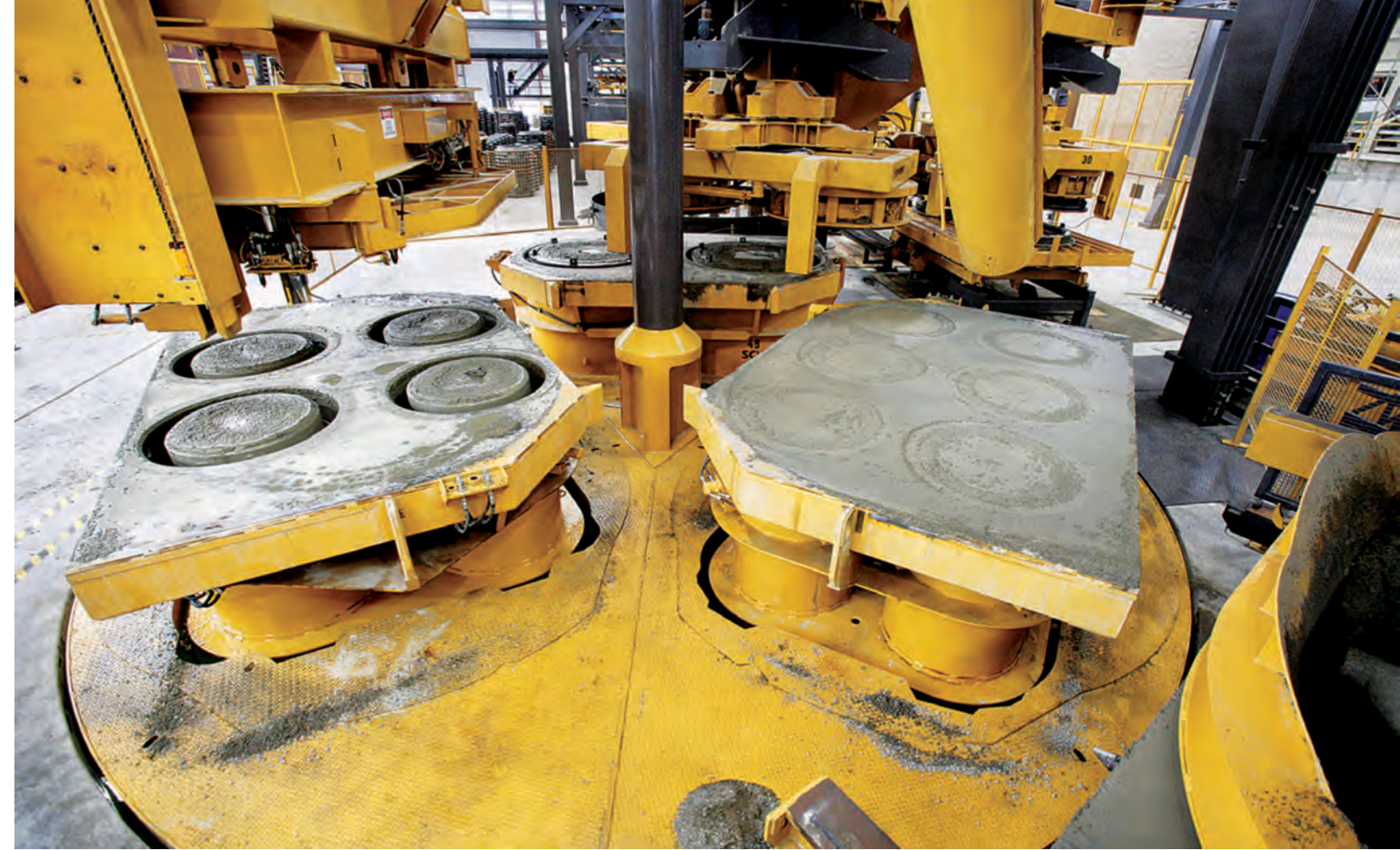
Automatic Crane Demolding
