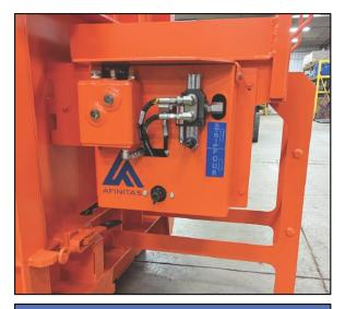
SmartConnect™ is mounted directly on the form to power the collapsible core hydraulics.
