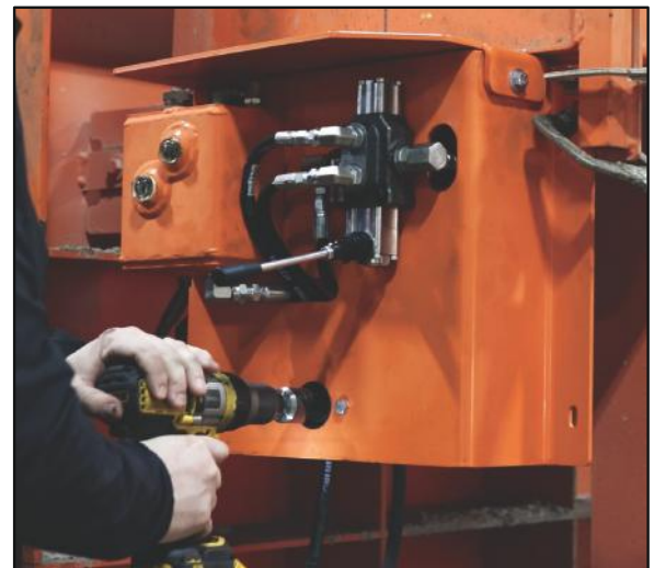
The self-contained unit is not dependent on any other equipment except a standard 20 volt - 1/2" drive cordless drill.
