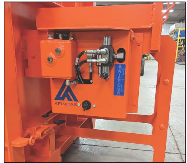
SmartConnect™ is mounted directly on the form to power the collapsible core hydraulics.
