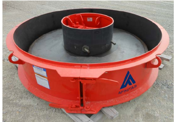
Slab Top Form
