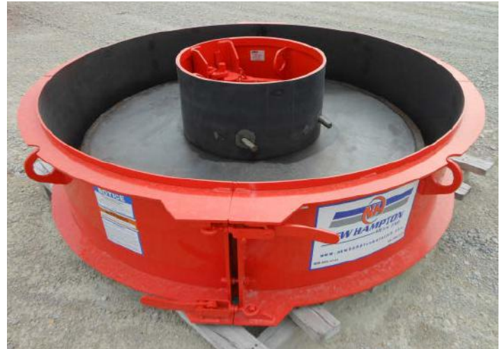
Slab Top Form
