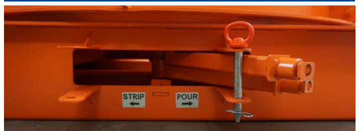
Quick Strip Sub-Base (Top lever controls manual step pin movement plus bottom lever controls manual core collapse)
