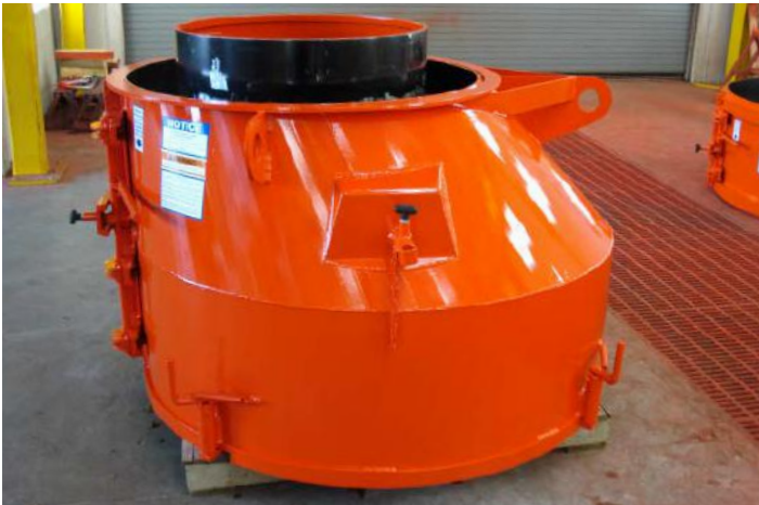
One Piece Form Design. Outward/Inward Facing Dog Houses. Dog Houses are used to provide sufficient concrete cover over lift inserts.
