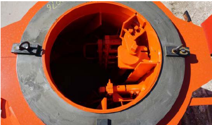
Hydraulic Core Collapsing with Hydraulic Step Pins Available Bolt Down Shovel Plate (Offered on Hydraulic Core Collapsing / Hydraulic Steps).
