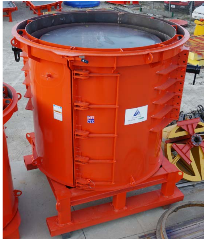
Riser – One-Piece (above) with Sub-Base Strip (below) and Optional Fork Truck Tubes
