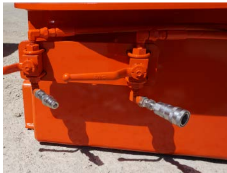
Hydraulic Core (outside view showing hydraulic connections)
