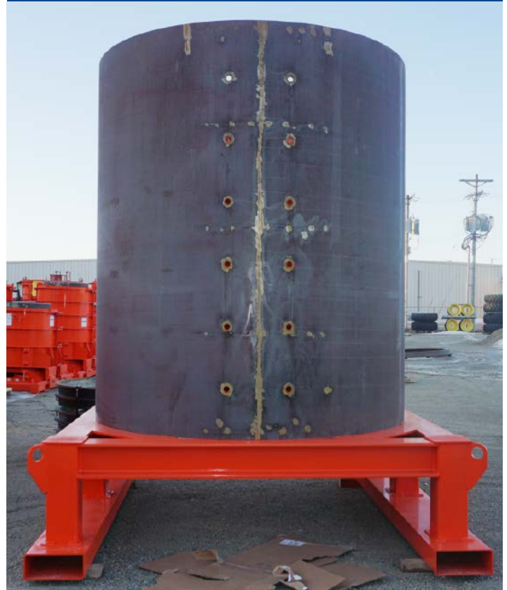
Riser – One-Piece (above) with Sub-Base Strip (below) and Optional Fork Truck Tubes
