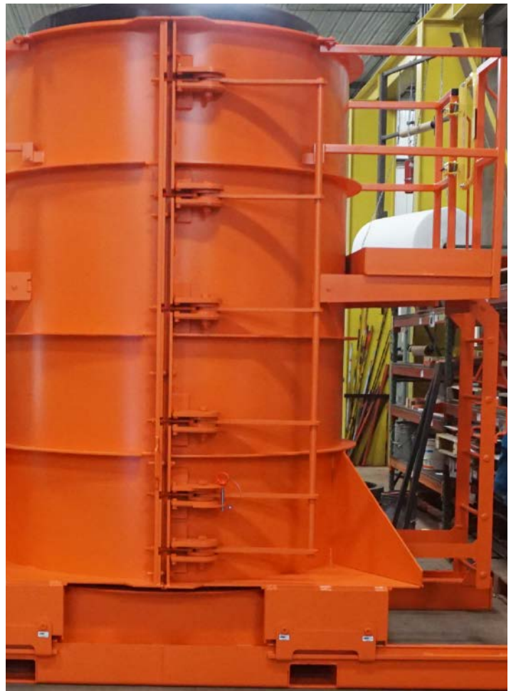
Ganged Form Latch Assembly for Two-Piece Forms and Roll Back Form Doors. Saves time opening and closing vs individual form toggle clamps, especially for taller forms where a ladder may be needed.
