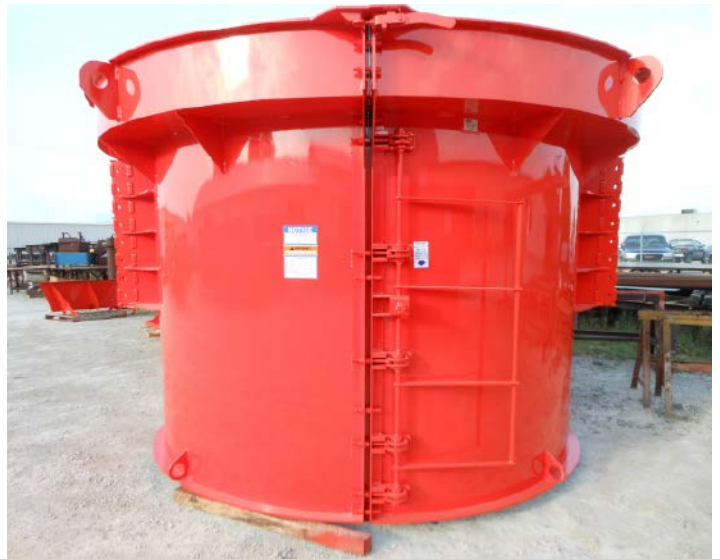
Manhole Base Form
