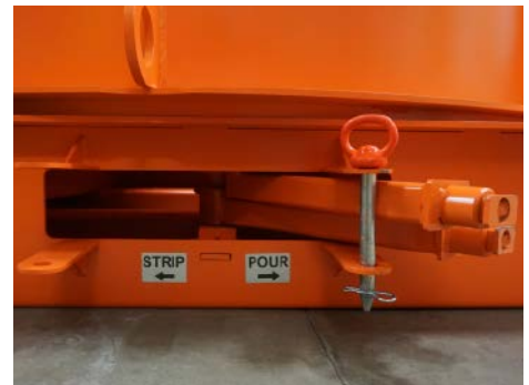
Quick Strip Sub-Base Top Lever Controls Manual Step Pin Movement Plus Bottom Lever Controls Manual Core Collapse
