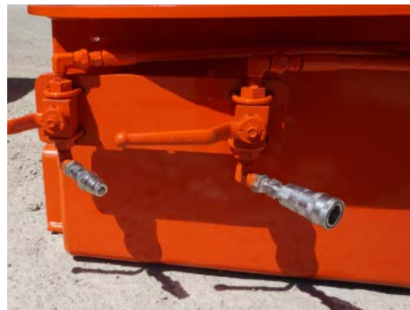
Hydraulic Core (outside view showing hydraulic connections)
