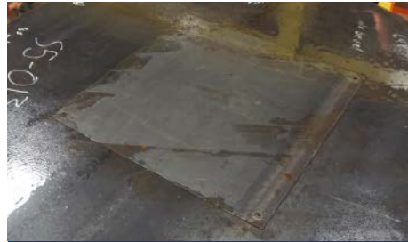
Option: Core Top Plate with Access Panel (Quick Strip)
