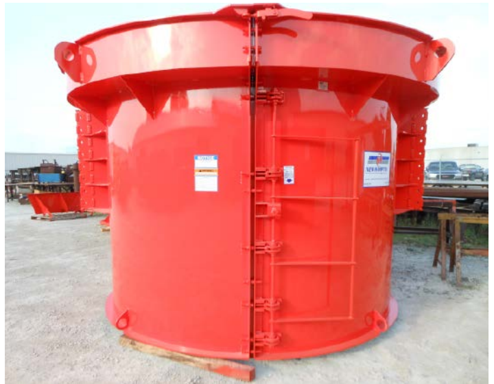
Manhole Base Form
