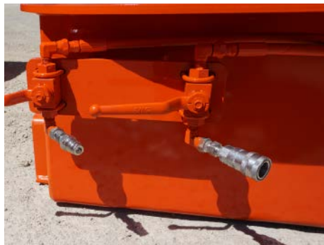
Hydraulic Core (outside view showing hydraulic connections)
