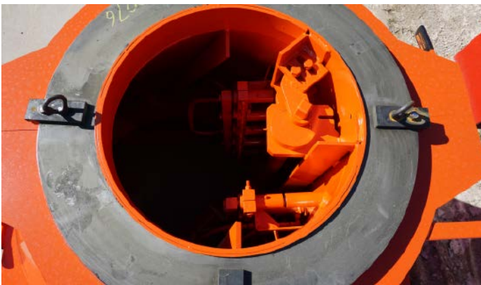
Hydraulic Core Collapsing with Hydraulic Step Pins Available Bolt Down Shovel Plate (Offered on Hydraulic Core Collapsing / Hydraulic Steps).
