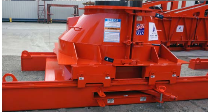
Roll-back Form Doors with Seam Flat Bars, Seam Alignment Pins and Pull Handles
