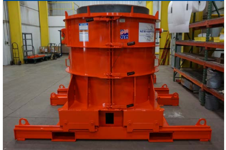
Quick Strip Sub-Base (Top lever controls manual step pin movement plus bottom lever controls manual core collapse)
