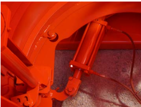
Hydraulic Core Collapsing (inside core view) 24" – 72" Diameter Cores with Quick Strip Sub-Base
