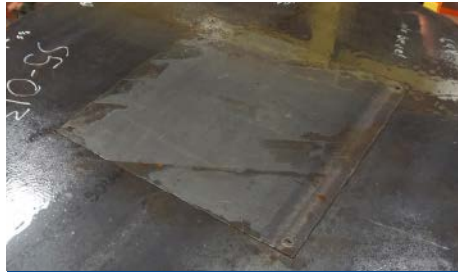
Option: Shovel Plate with Access Panel (Quick Strip)
