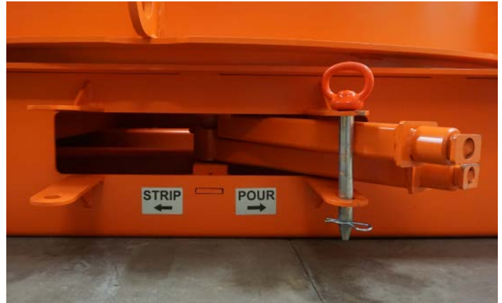
Quick Strip Sub-Base (Top lever controls manual step pin movement plus bottom lever controls manual core collapse)
