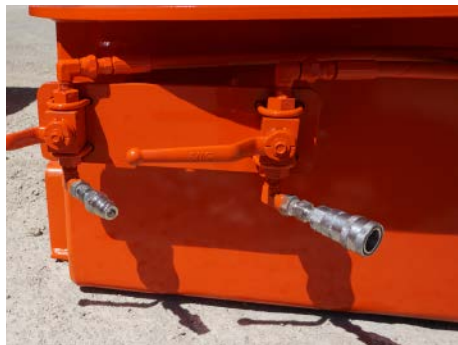
Hydraulic Core (outside view showing hydraulic connections)
