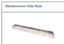
Weckenmann side rails are primarily paired with Weckenmann architectural self-stressing flat slab beds and have various other uses in automated and semi-automated plants. The laser cut side rails, made in a robotic welding jig, have extremely tight tolerances. Base rails are typically 6 or 8 inches high and come with integrated magnets. Risers of 2, 3, or 4 inches and chamfer can be added to fit customers' requirements. Made in Germany
