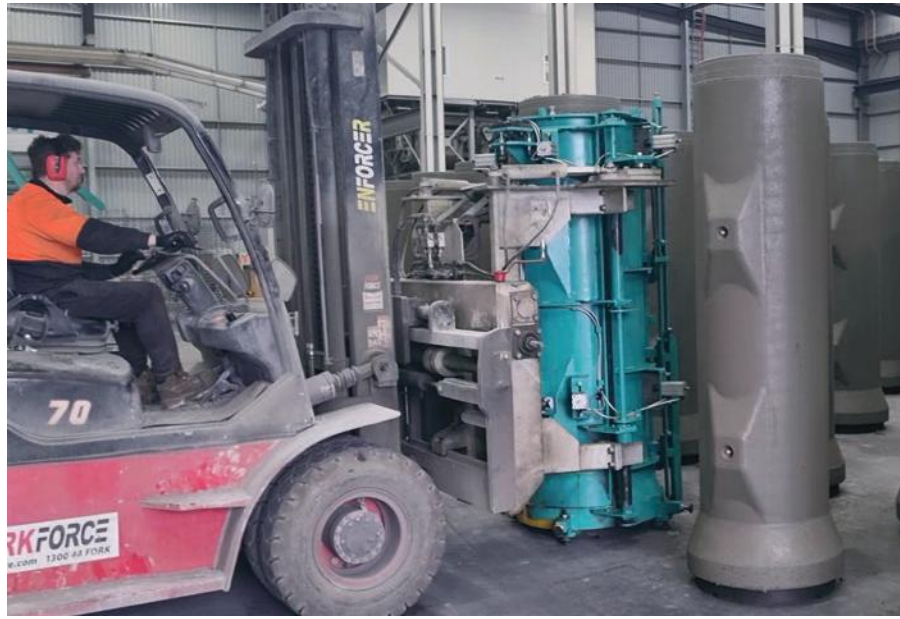
Three-piece mold design with forklift truck demolding device.
