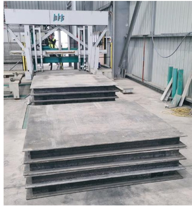
The Atlantic 1515 with pallet handling on the right side. The pallet magazine is adjustable to accommodate a range of pallets.
