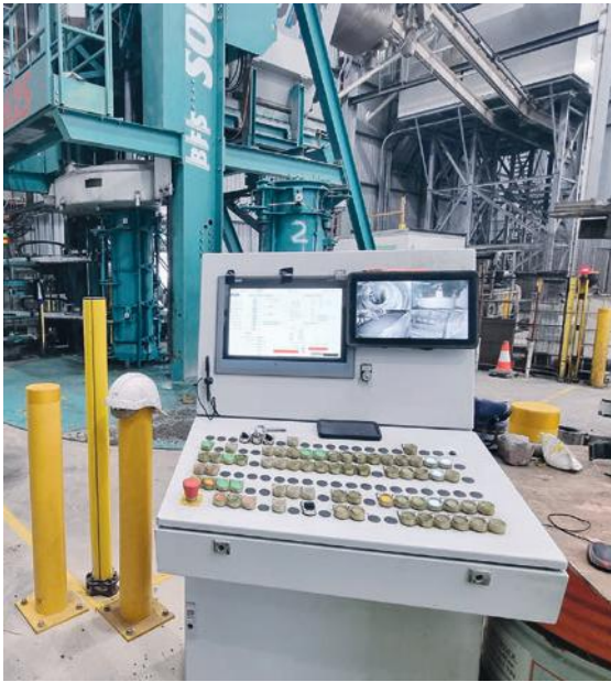
Souveraen's computer-controlled production and camera system.
