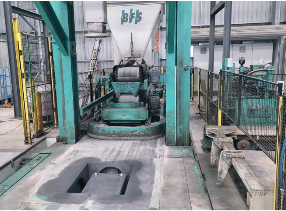
The Atlantic 1515 with pallet handling on the right side. The pallet magazine is adjustable to accommodate a range of pallets.
