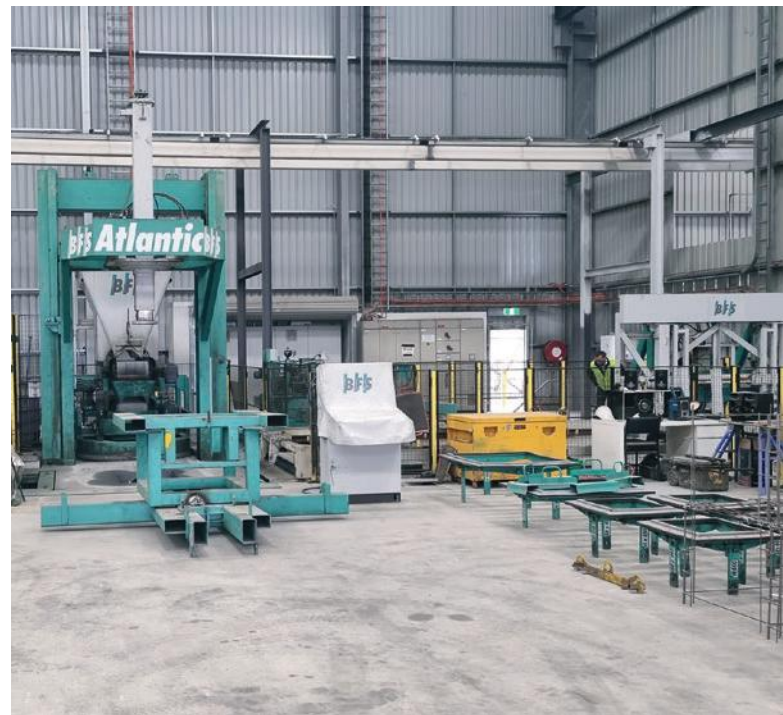
Frankston's BFS Atlantic 1515 system is designed to produce tanks, pits, manholes, tapers, pipes and similar concrete products with a height up to 1500mm and a max inner diameter of 1500mm and square products up to 900mm x 900mm.
