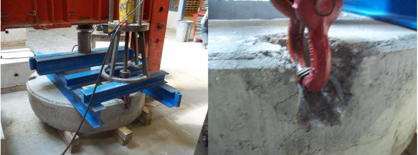
Figure 1 – 90-degree Tension Test Set-up
