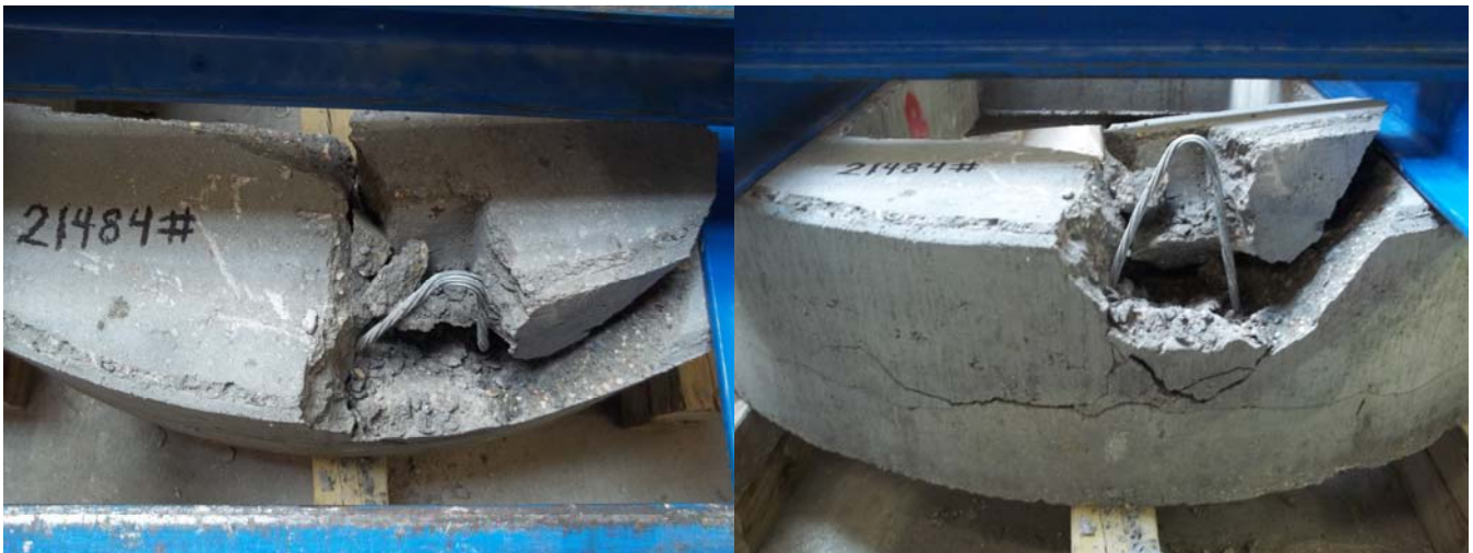
Figure 2 – Tension Failure Mode
