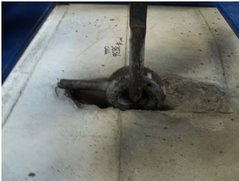
Figure 1 – 90-degree Tension Test Set-up
