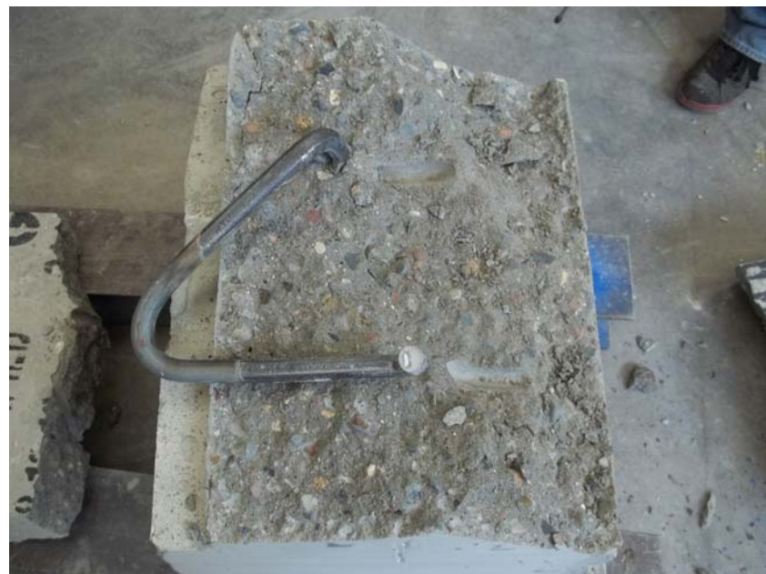
Figure 2 – Tension Failure Mode
