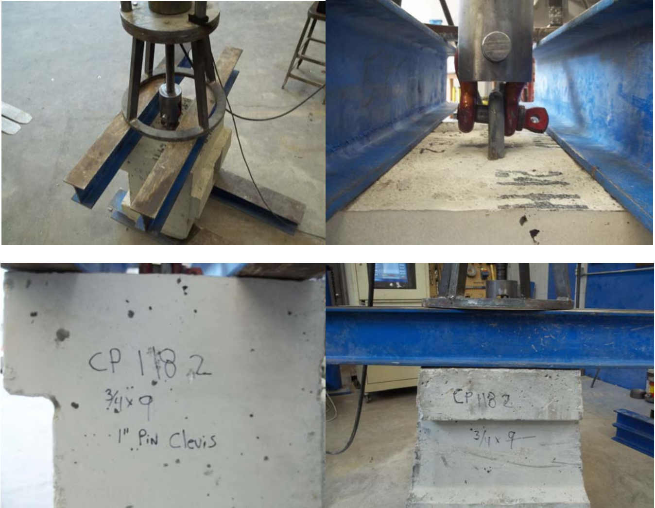
Figure 1 – 90-degree Tension Test Set-up
