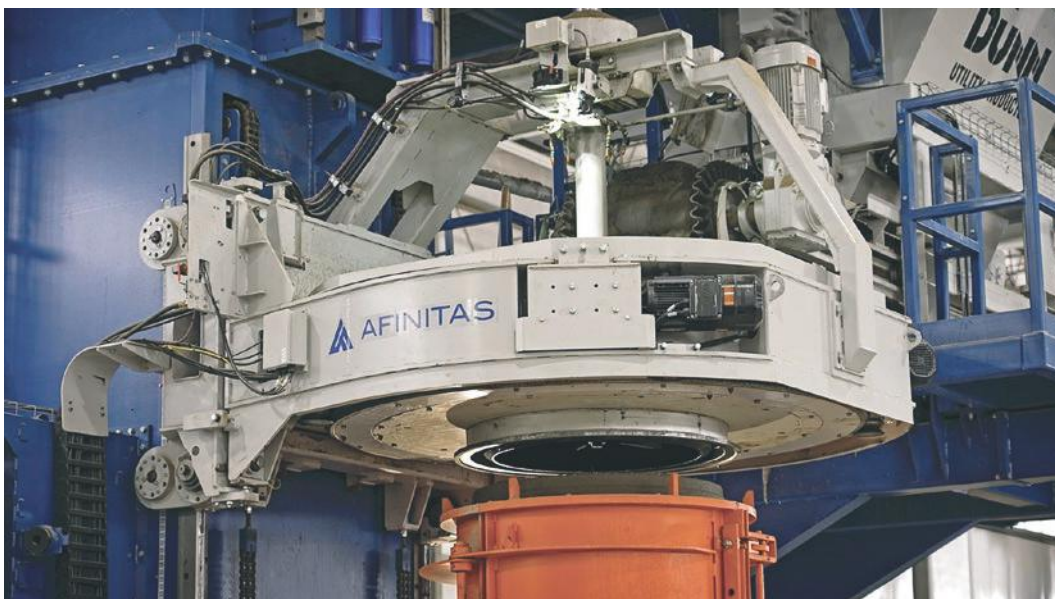
ePak's powerful rollerhead drive
