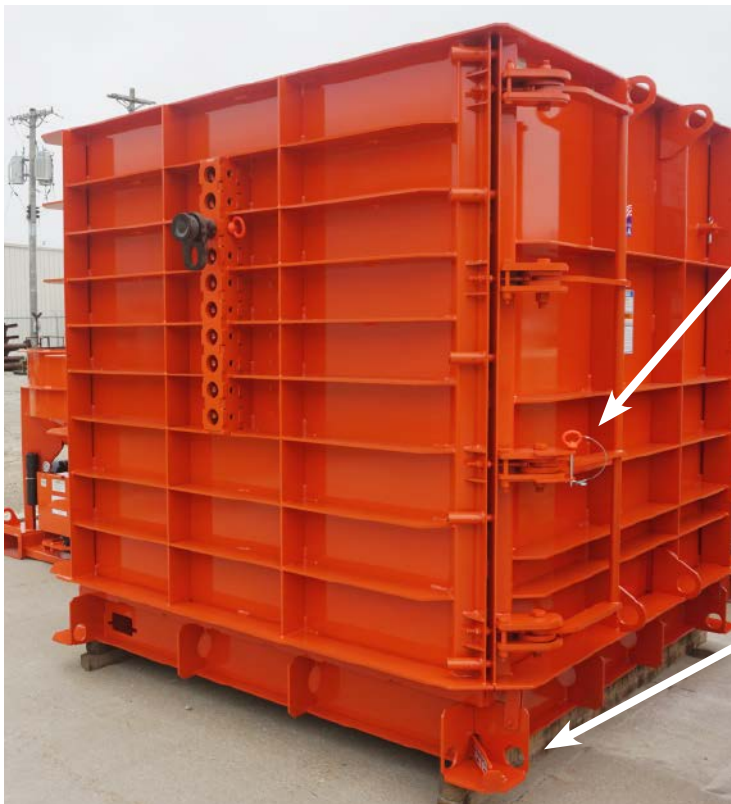
Ganged Form Latch with Open/Close Lock
