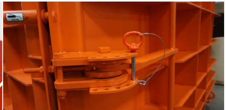
Ganged Form Latch with Open/Close Lock
