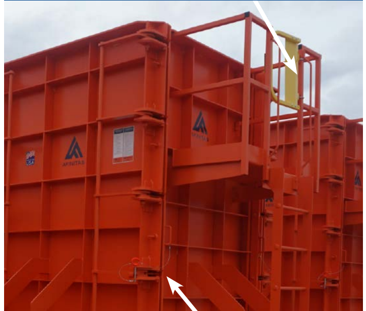
Ganged Form Latch with Open/Close Latch Lock Saves Time Opening and Closing vs. Individual Form Toggle Clamps, Especially for Taller Forms Where a Ladder May Be Needed
