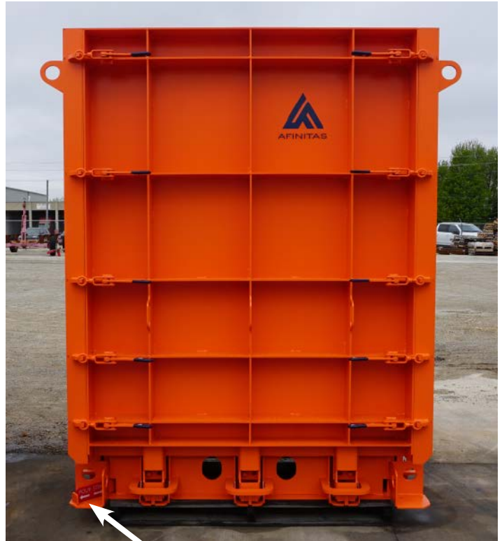
Bolt Down, Beveled Core Top with Access Panel (Important feature for easy access to maintain the inner core corners)
