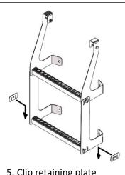
5. Clip retaining plate over lower rung
