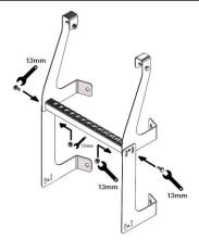
3. Secure stringers with M8x16 bolt and nut. Ensure rung is secure.
