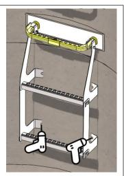
8. Secure ladder to manhole. Do not add additional rungs.
