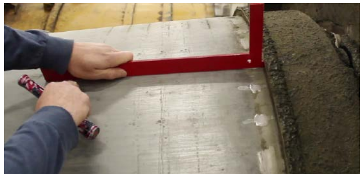
Core bottom wear and seal band inspection
