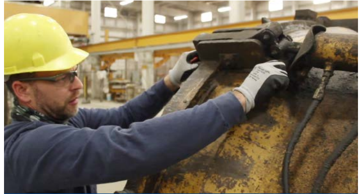
P-Lock assembly inspection
