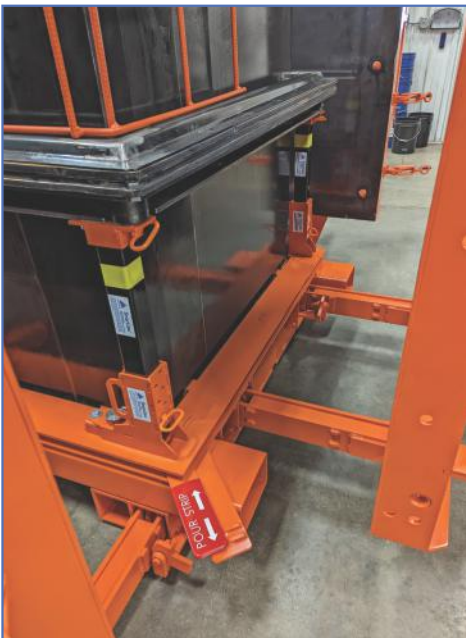
SmartJax™ pallet support on box form.
