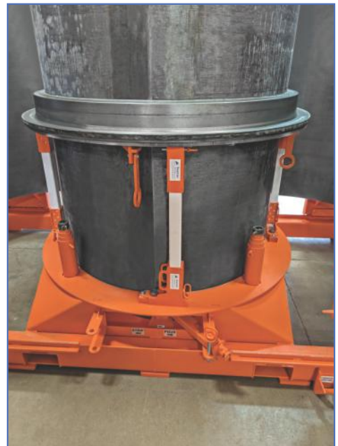
SmartJax™ pallet support on round form.
