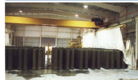
Canopy Kiln – The traditional solution for curing various concrete products.
