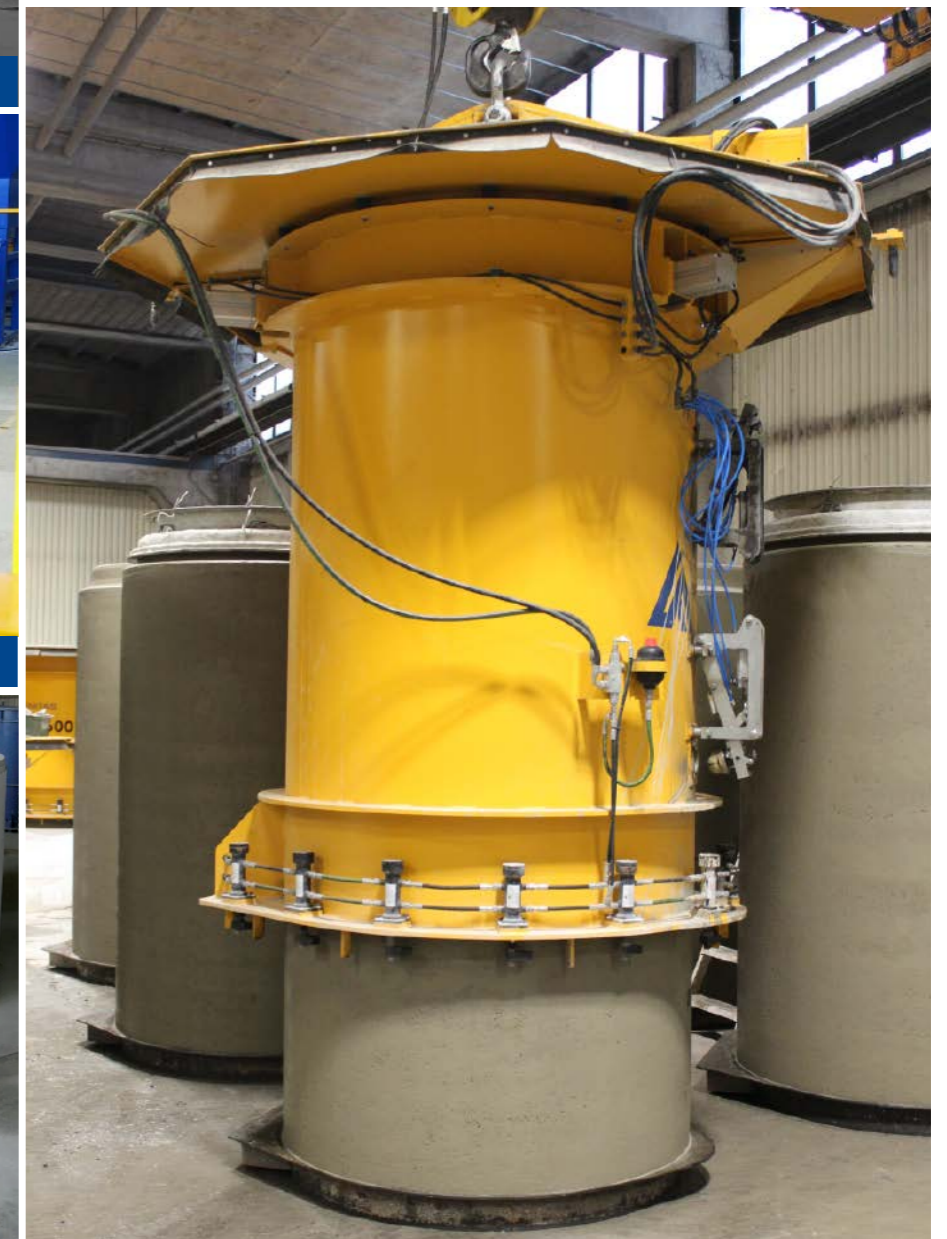
Product demolding with hydraulic pallet clamps
