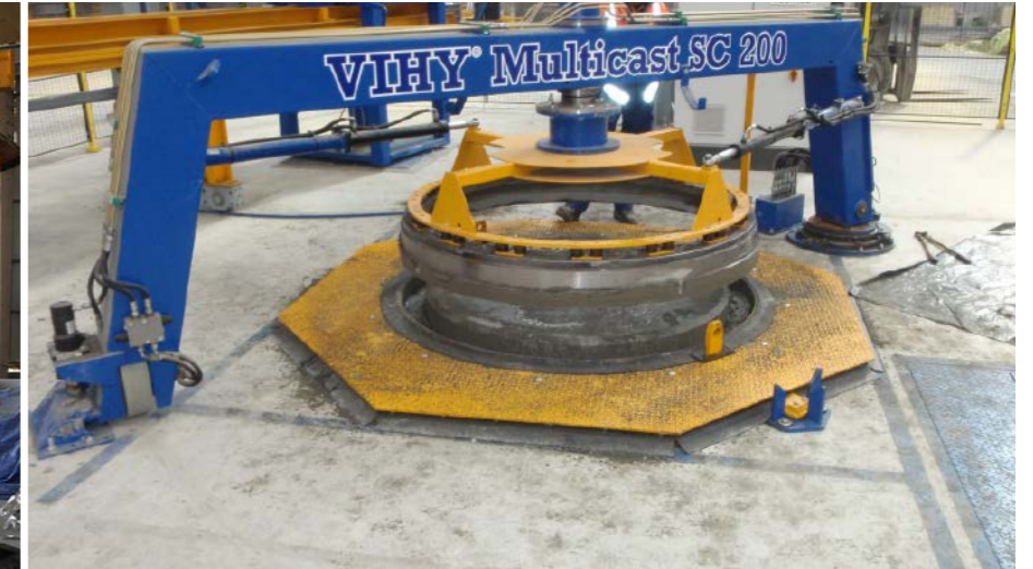
Spigot forming by hydraulic-driven press
