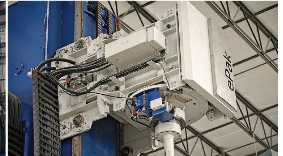
Unique gearless, electronic drive
