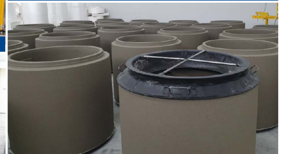
Manhole finished product
