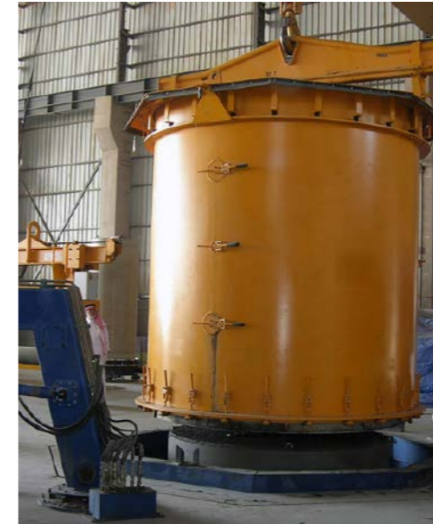
Spigot forming by hydraulic-driven press
