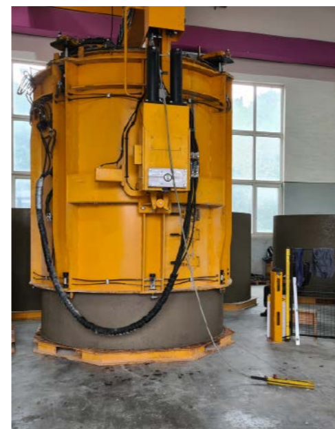
Filling and vibration of base section
