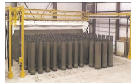
Telekiln – The simple and quick method for covering concrete pipe and manholes.
