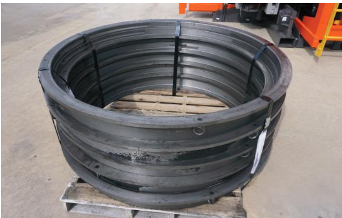
Tongue Forming Pallets with Lifting Eyes
