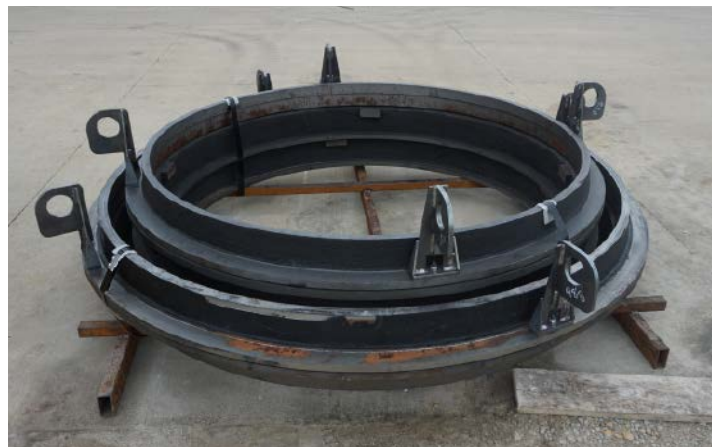
Tongue Forming Headers, Open Top with Form Hangers/Lifting Eyes
